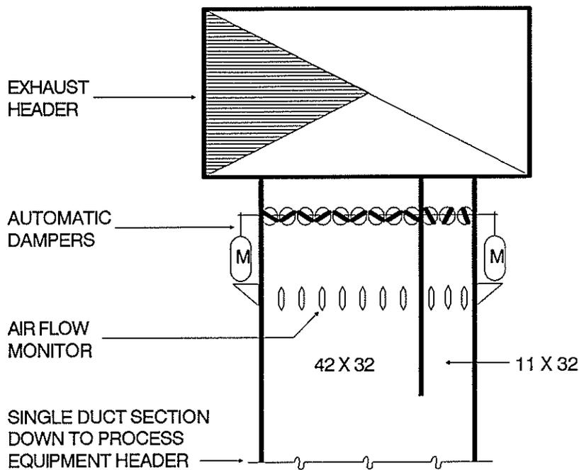
Fig. 2. Section view of zone damper and monitor.
