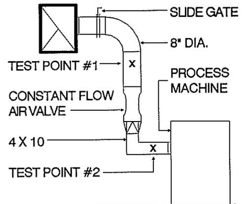
Fig. 1. Duct-pressure tests.
