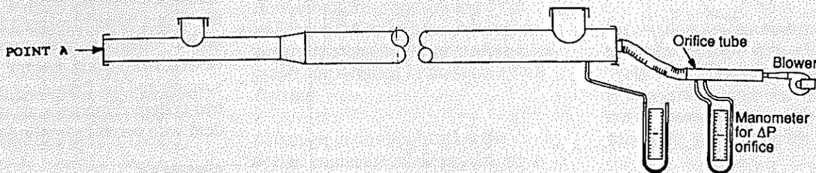
Fig. 1. A typical duct-leak test setup.
