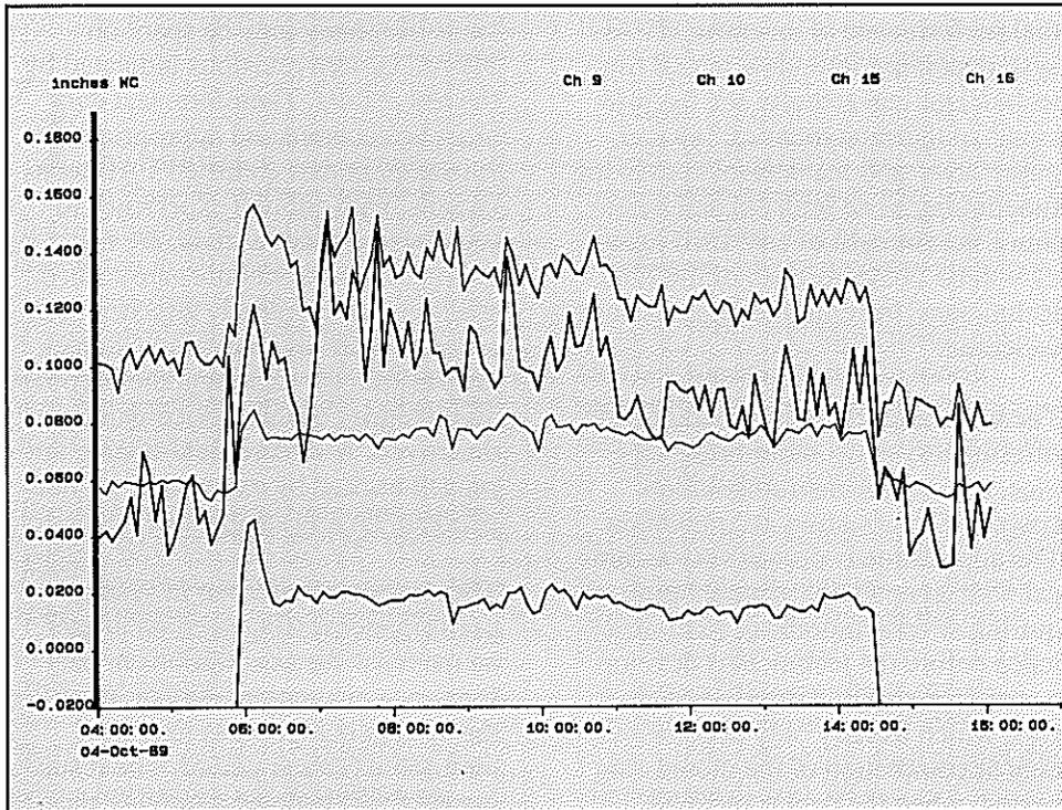
Pressurization hierarchy for the four areas pictured above, during a period when a construction door was left open. Atmosphere reference is aero.
